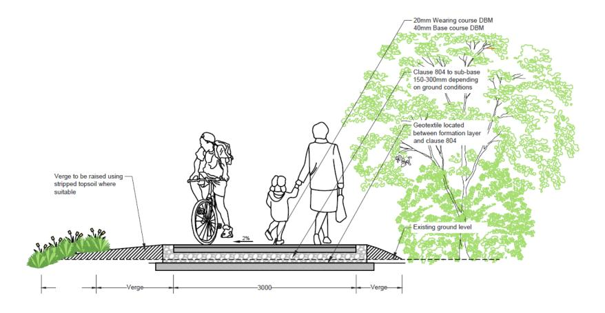
TYPICAL BOUND SURFACE (Approach to road crossings 10m either side) SCALE 1:25
