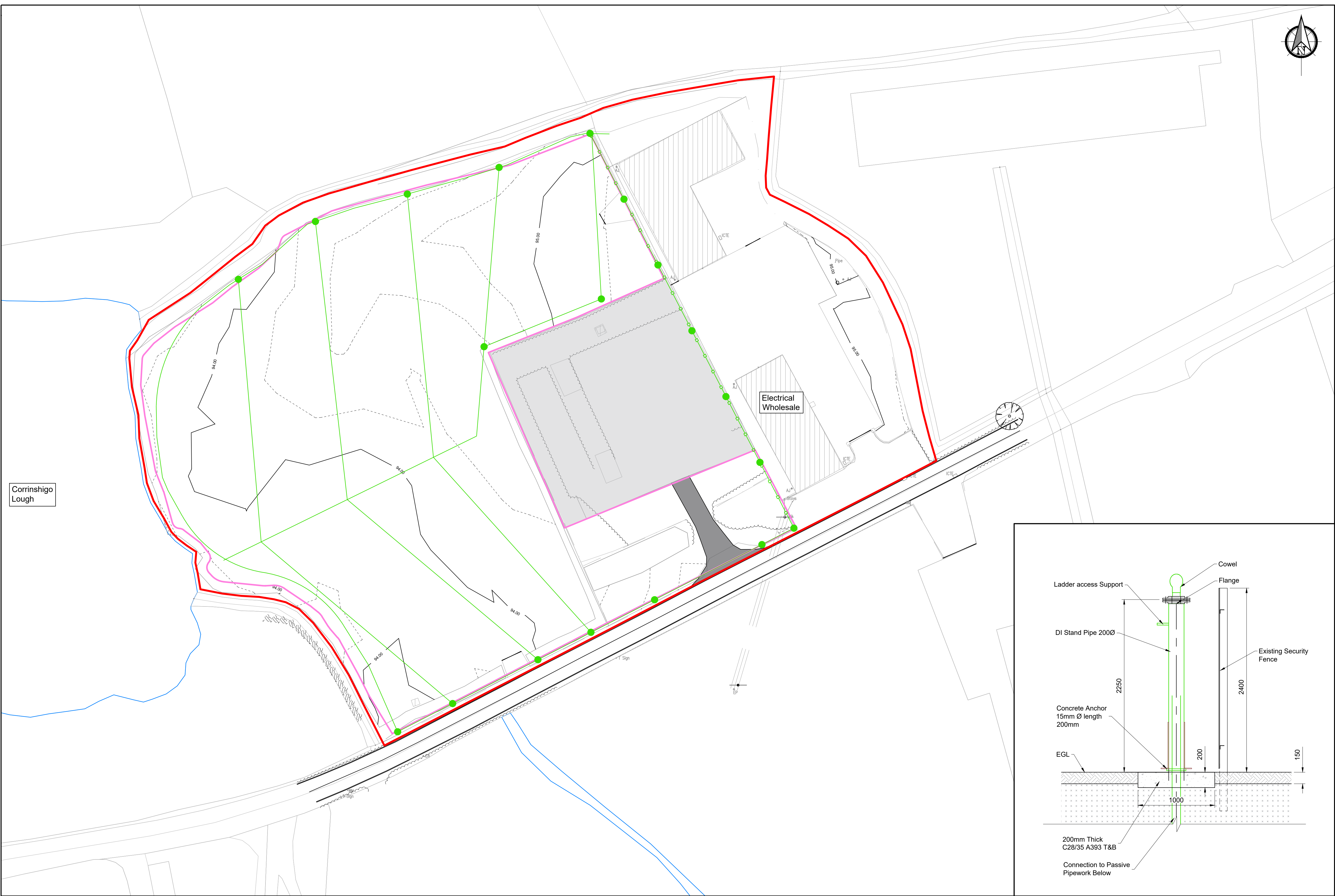
PASSIVE LANDFILL GAS VENTILATION STAND PIPE TYPICAL DETAIL
