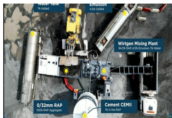
Figure 16 - Mobile Rap Plant set up in Co. Monaghan
