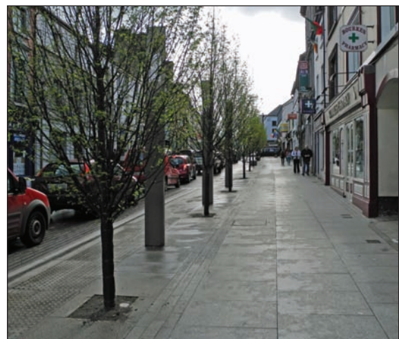
Figure 4.33: Example from Castlebar, Co. Mayo, where the verge acts a designated space for street furniture, lighting facilities and planting of trees, keeping the footway clear of obstacles.
