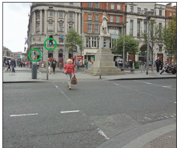
Figure 4.39: Example of a wide streets with a crossing that allows pedestrians to cross in a direct manner and in a single movement. The median acts as a refuge island for those users who cannot cross the street in a reasonable time.
