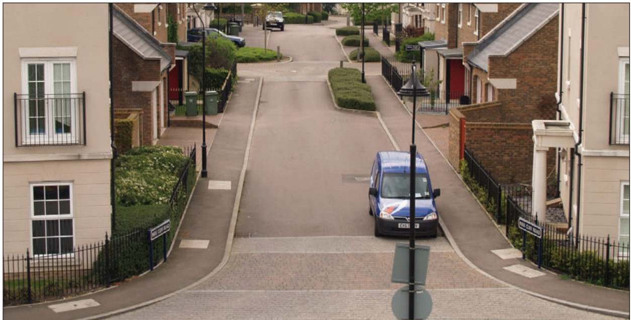
Figure 4.71: An example from Ingress Park, Kent, UK, of how the path and speed of a vehicle is altered within a low speed environment through the use of vertical and horizontal deflections (and material changes).
