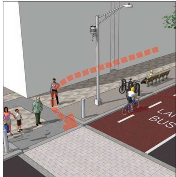
Figure 4.19: Items such as a bicycle racks, seating and/or bollards are less intrusive elements that can be used to guide pedestrians toward crossing points and reduce illegal kerb mounting.
