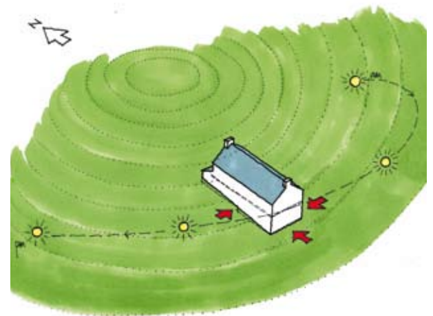
Modestly sized two storey house with long axis at a right angle to contours
