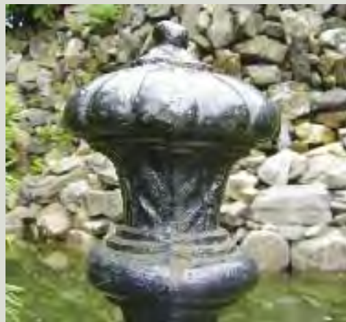
Castings should be checked before they are put in place to ensure that they are of acceptable quality. The casting illustrated above is deformed because the two halves of the mould were not aligned correctly during the casting process
