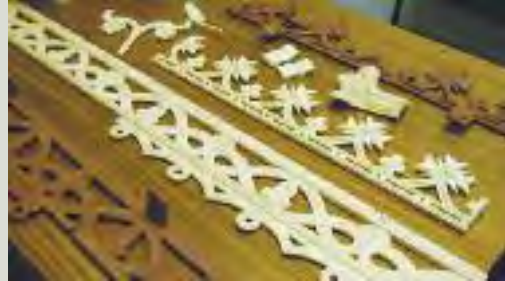
It is advisable to inspect patterns before they are used for making castings to ensure that the detailing is accurate and that the surface finish is smooth (Image courtesy of Historic Scotland)
