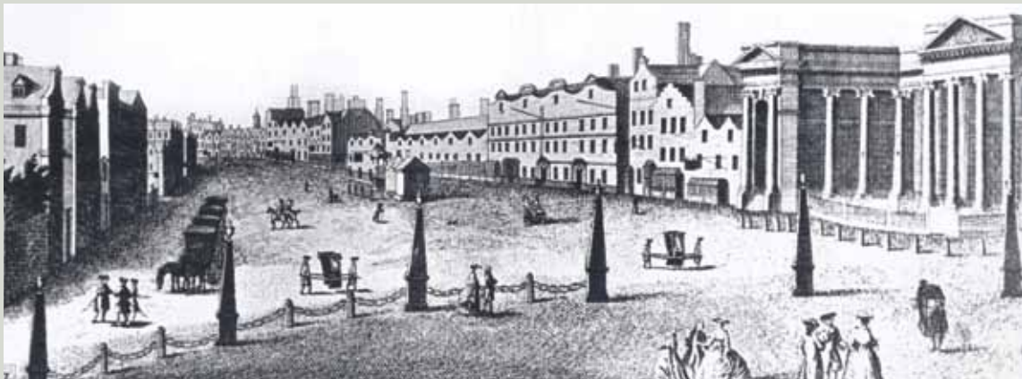
A Prospect of the Parliament House, in College Green Dublin by Joseph Tudor, 1753. In Ireland and Britain, as in continental Europe, the construction of footpaths separated from the general carriageway did not begin to emerge as the norm in city streets until the eighteenth century. This view of College Green shows the street paved as a continuous surface with no footpaths, and with bollards enclosing areas in front of Trinity College and the Parliament House. Tudor's view of Sackville Street and Gardiner Mall in the same decade shows footpaths in this new development, but not on the existing side streets: Henry Street and Earl Street
