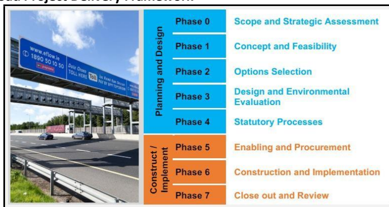
Figure 7.10: TII Road Project Delivery Framework
