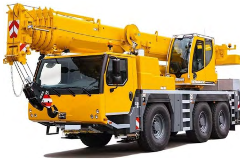
Figure 4-3 – Typical mobile crane for 400 kV tower erection
