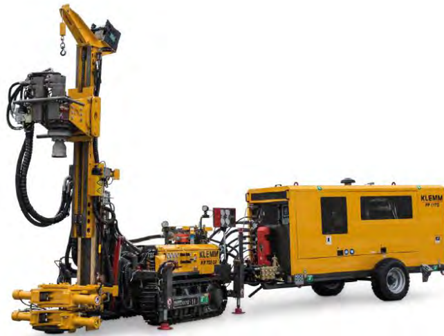
Figure 5-4 – Typical mini pile rig
