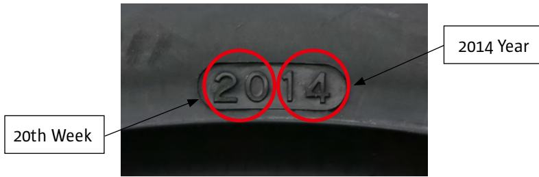
Figure 7: Production Date Code 2014 = 20th week of 2014
