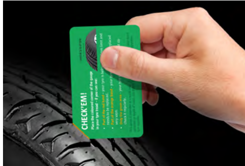
Figure 5: How to use the handy pop-out tyre tread depth gauge.
