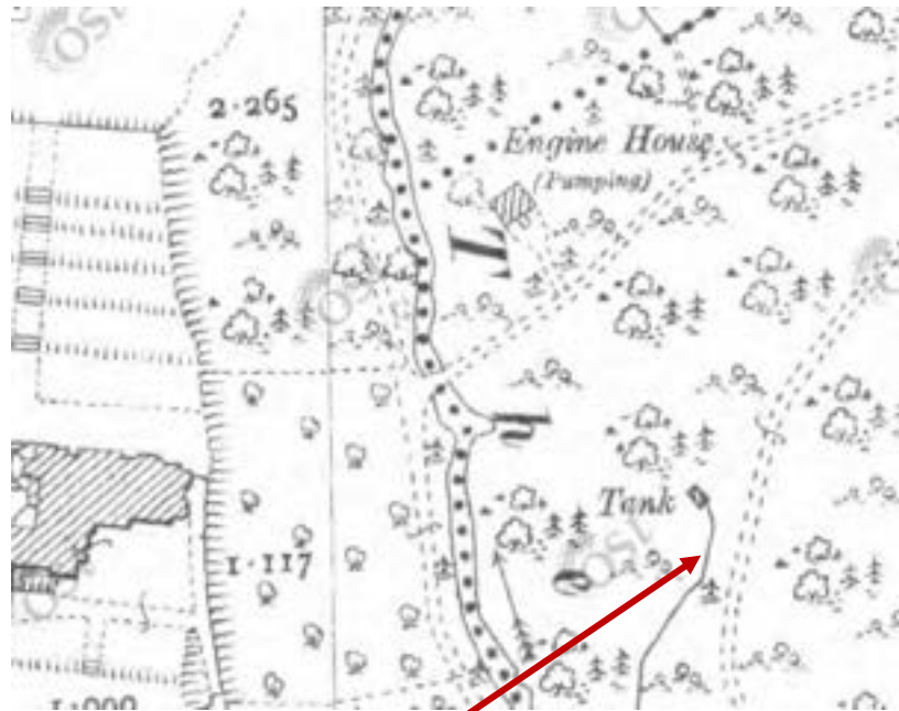
Feeder pipe to the Engine House from the Tank is not shown on Historic 25" OS map. The mill race from the stream to the tank is indicated with a line. Rossmore Castle is to the southwest of the Engine House.
