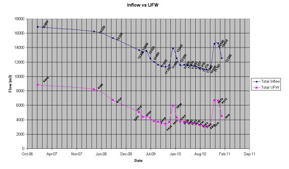
Conservation Project has now established active leakage control on all 54 DMA's (District Meter Areas). UFW currently standing at 36% (Please note this figure was as low as 28% before the big freeze)
