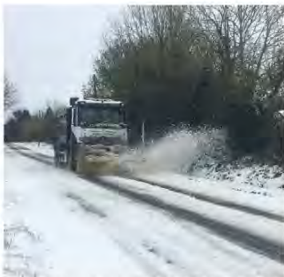
Snow plough in operation on regional route
