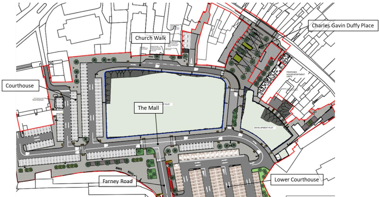
Figure 9.11 – Proposed Internal Street Network and Alignment
