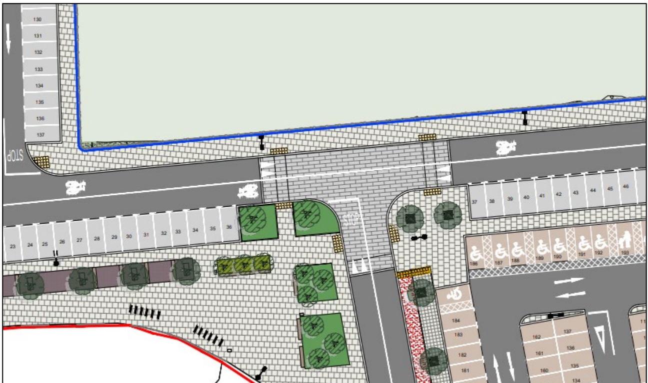
Figure 2.23: Excerpt from Planning Drawing 231932_DSS_OP_G_101 showing the proposed Mall and connection to Farney Road
